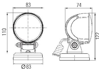
**Module 70 with magnetic base and spiral cable**
